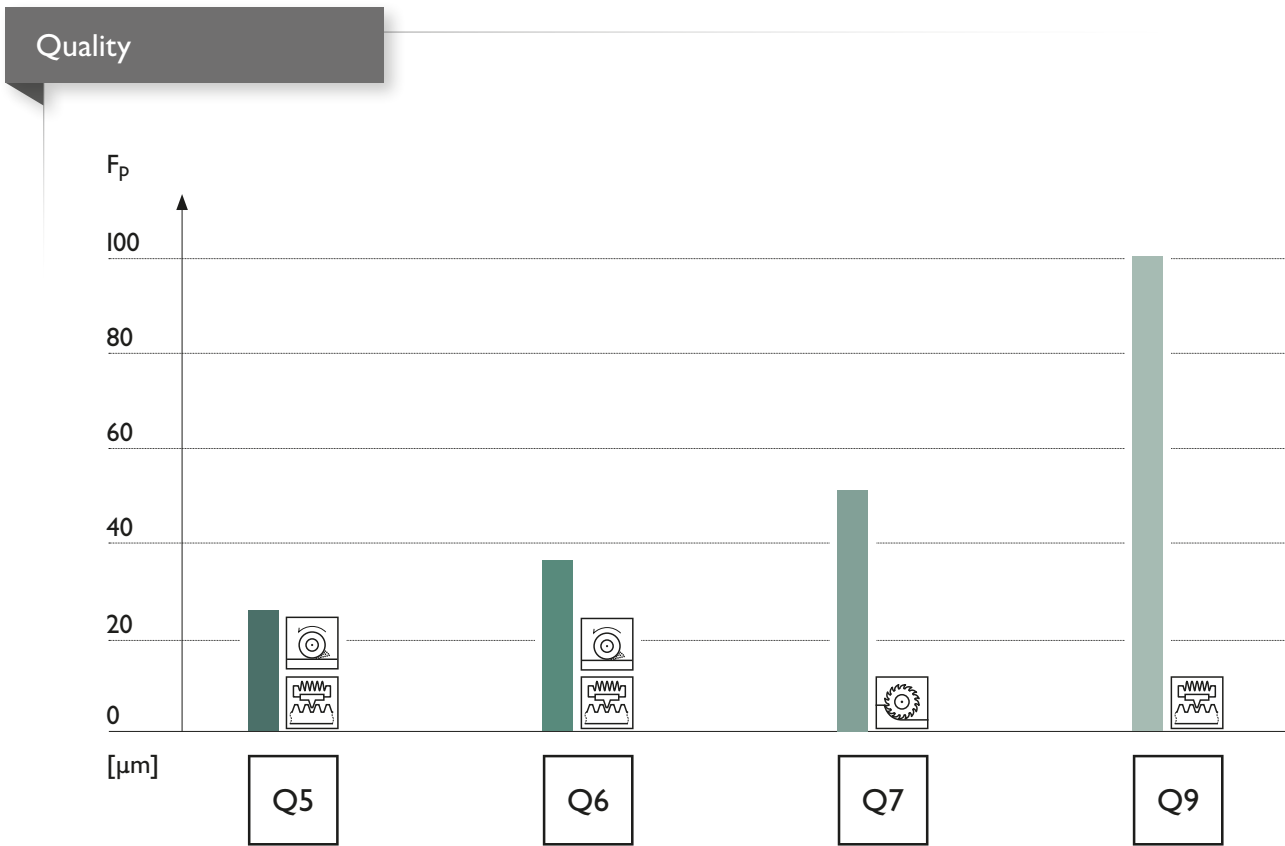
Example of the cumulative pitch deviation F_p for module 4 based on length 1000mm. Quality DIN 3962.
